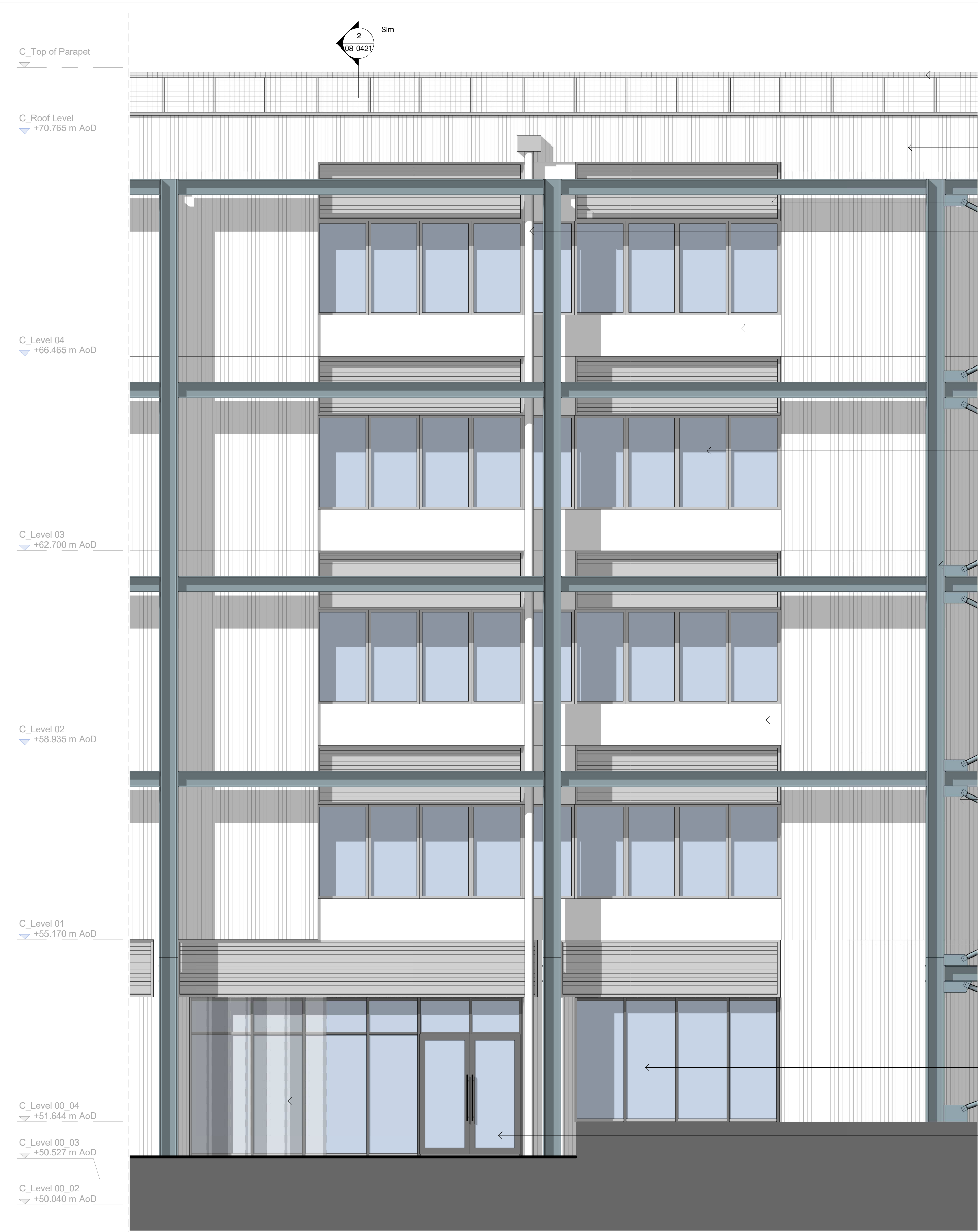
Building C - Bay Elevation 02 1 : 50
