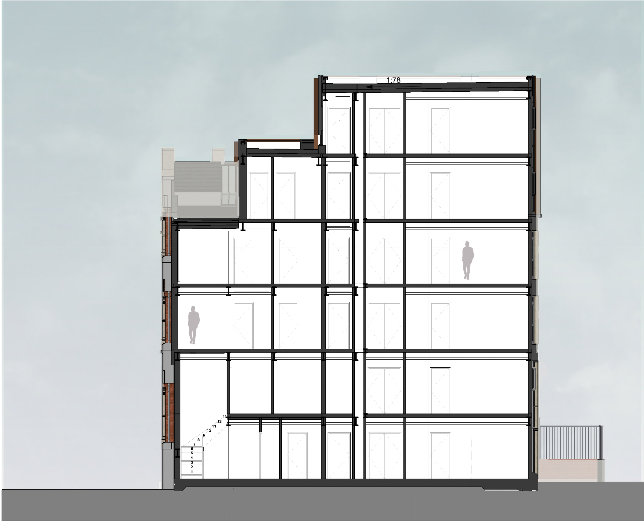
Cross Section B - Proposed 1:100
