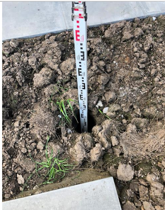
Depth of Cover System at Ground Level
