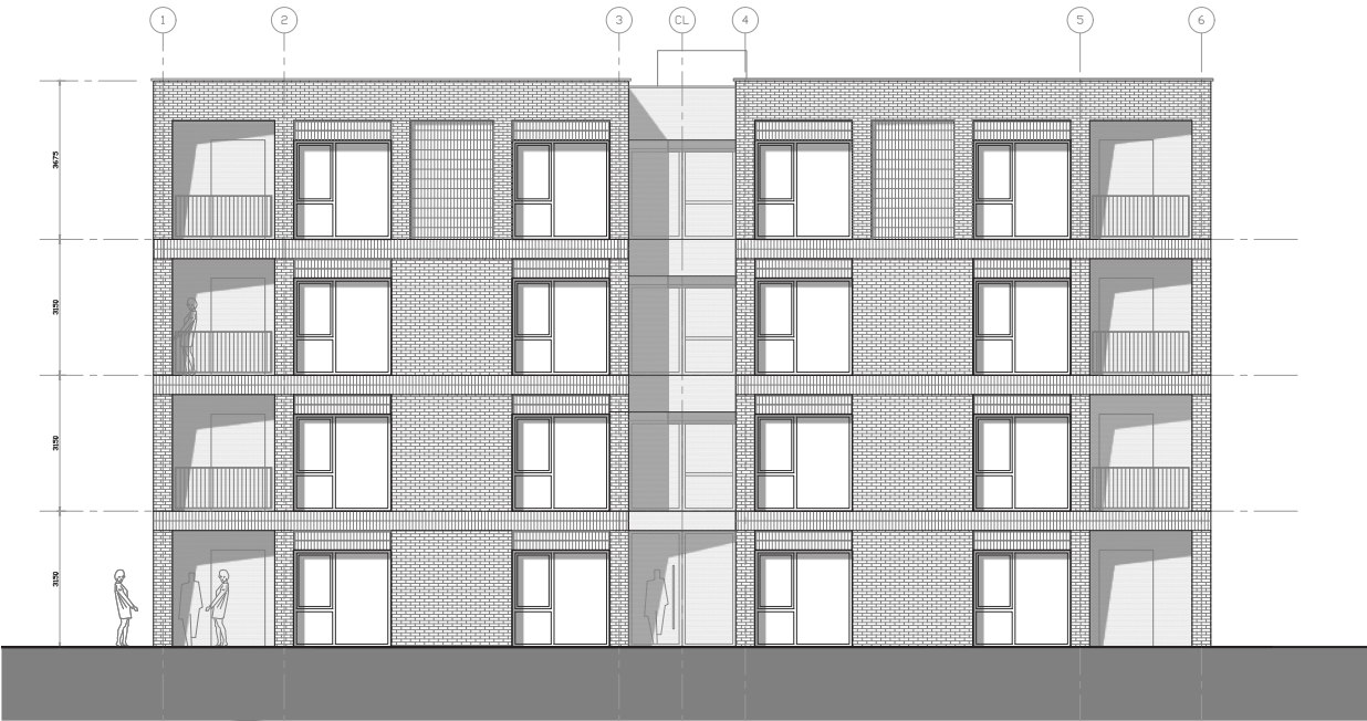
Front Silk Street Elevation - Main Entrance
