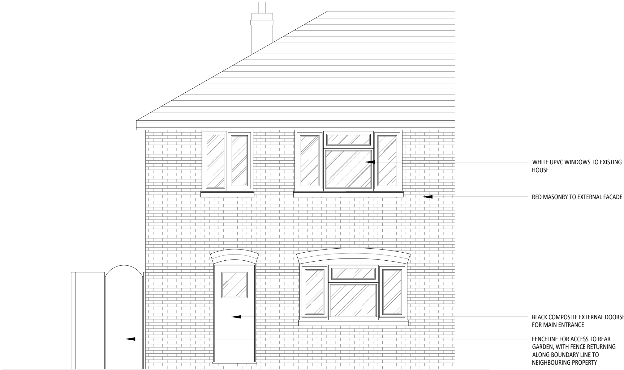
04 000 EXISTING REAR ELEVATION SCALE - 1:50@A1 ELEVATION
