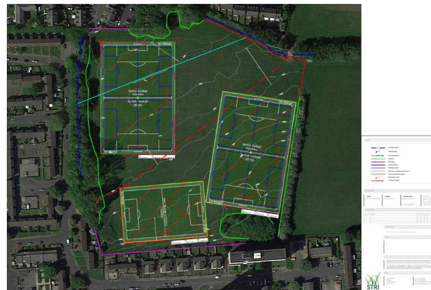
Figure 4: STRI Earthworks calculations for the proposed pitch layout within Wythenshawe Park.
