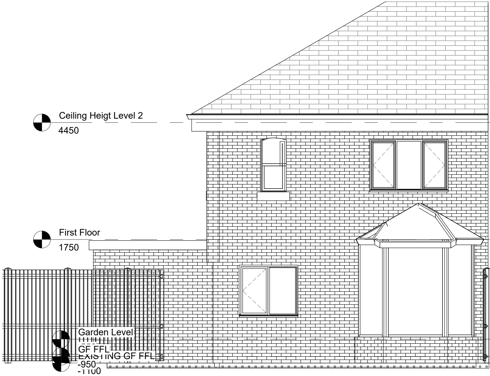
2 EXISTING SOUTH ELEVATION 1 : 50
