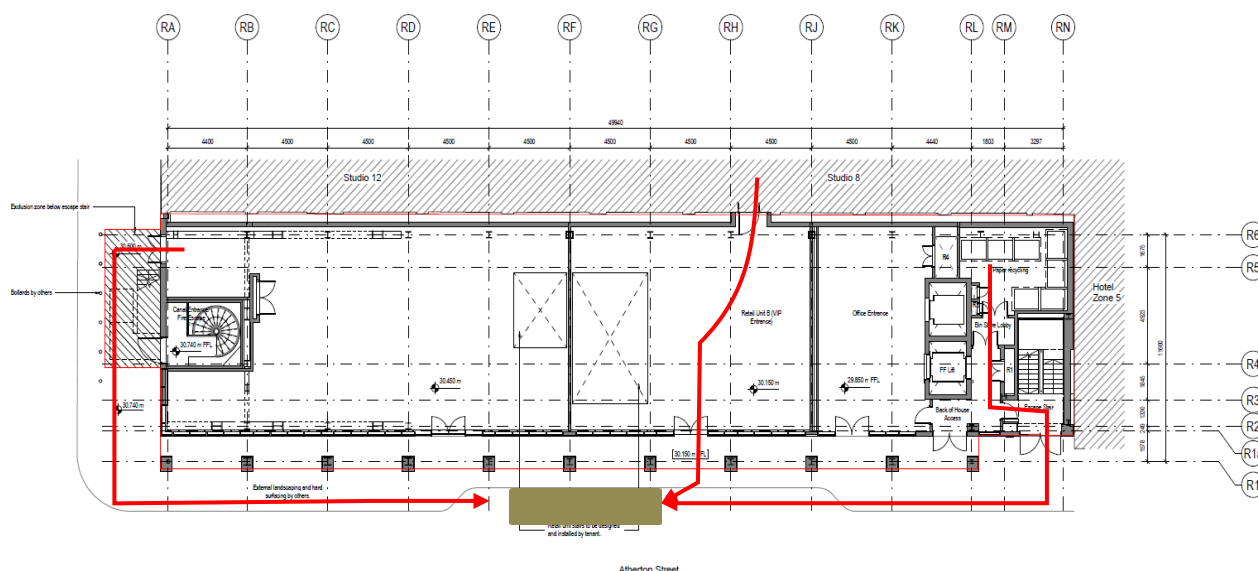
Figure 3.2: Bin Store Provision & Routing – Zone 6 Ground Floor
