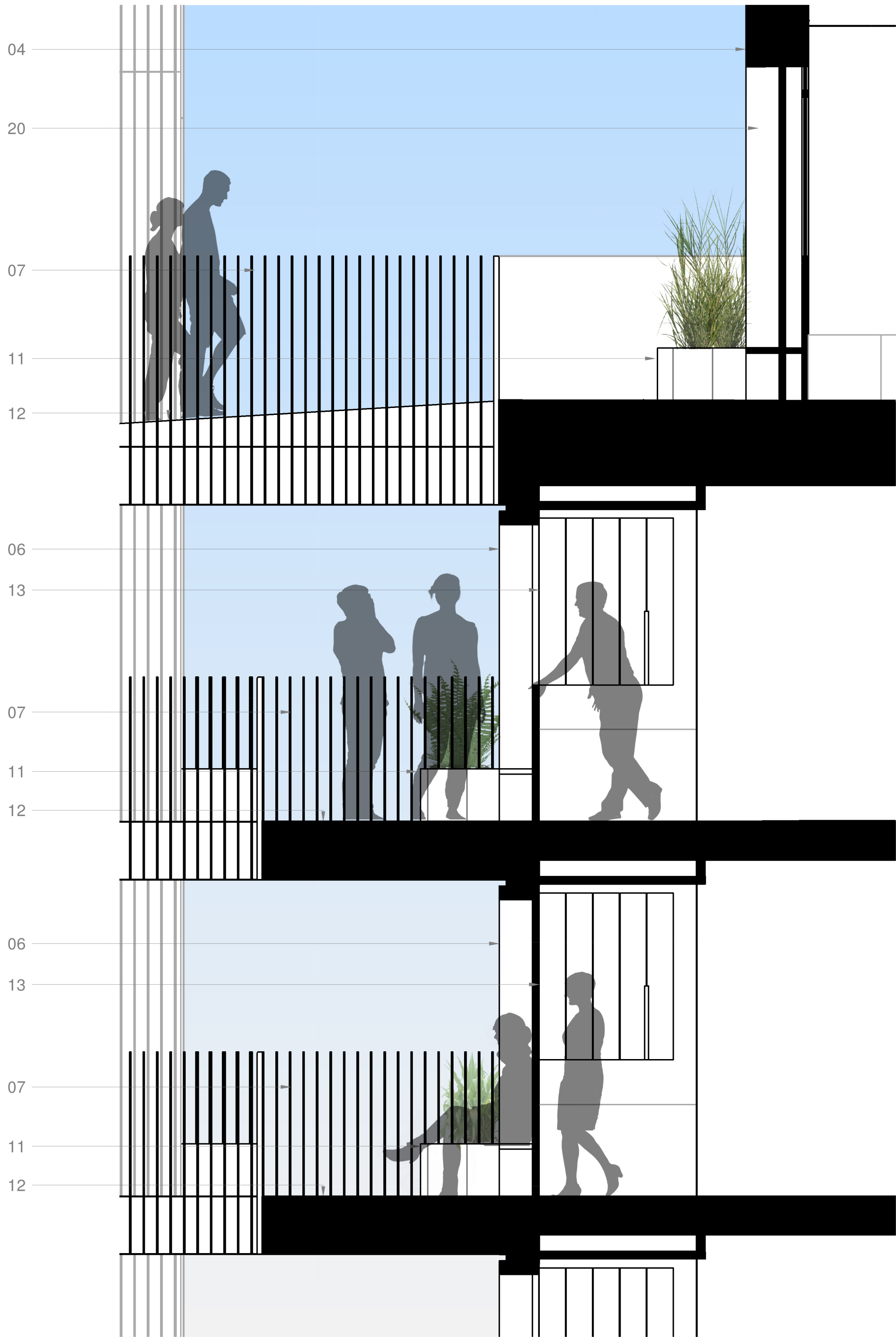
2 Section - Internal Courtyard - Level 08-09 1 : 25
