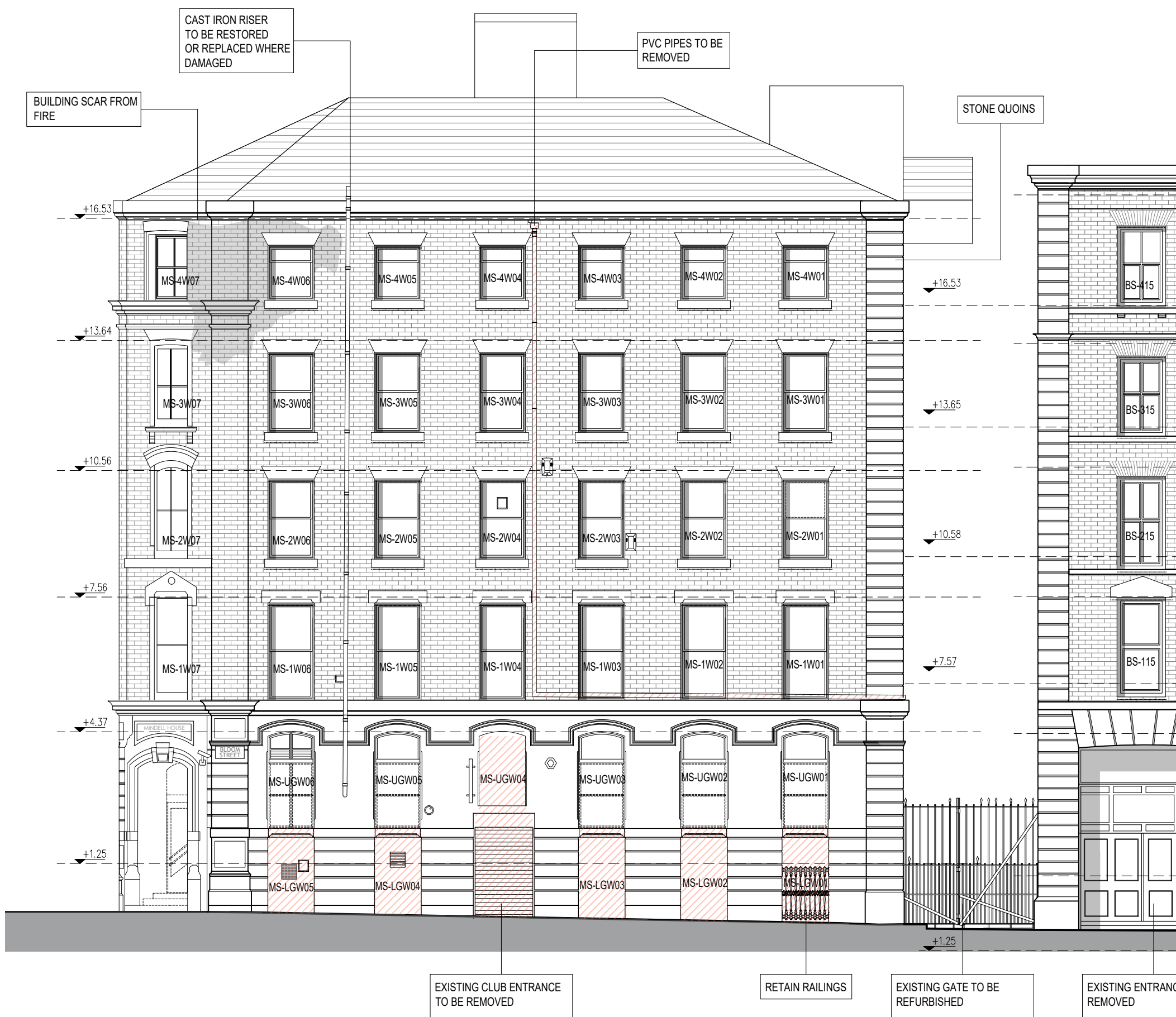
Existing - Mindel House Existing elevation - 04 Scale 1:100 @ A1
