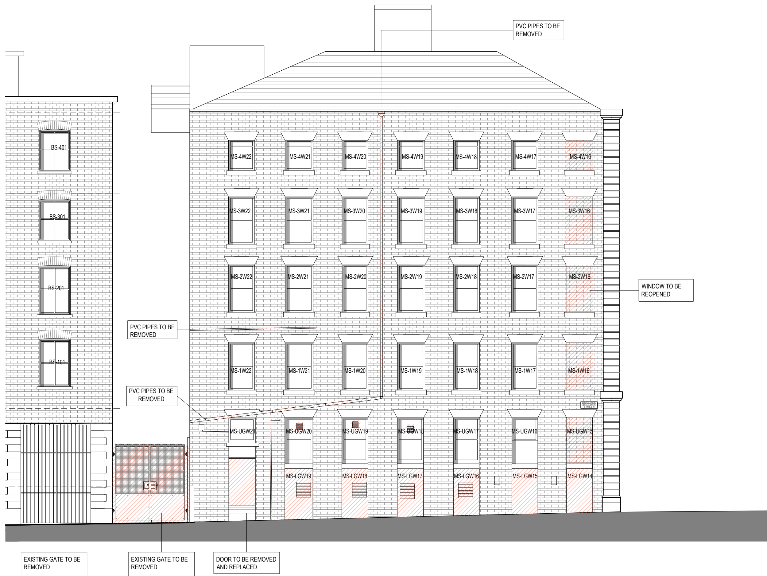
Existing - Mindel House elevation - 02 Scale 1:100 @ A1
