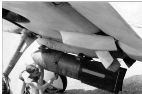
SC250 attached to undercarriage of Messerschmitt Bf109
