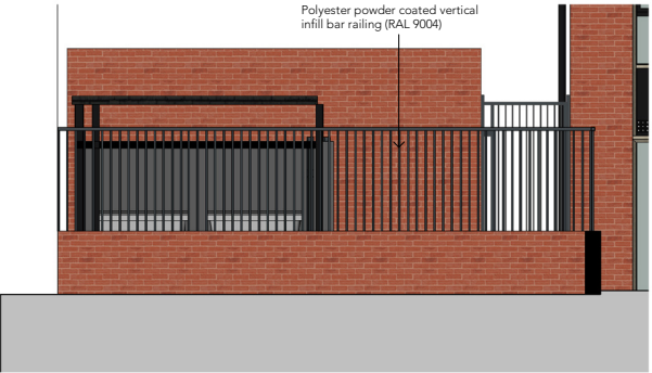
Bin and Bike Store South East Elevation 1: 50
