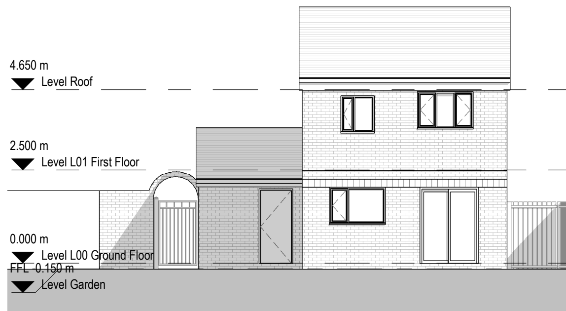
3 Existing East Elevation 1 : 100
