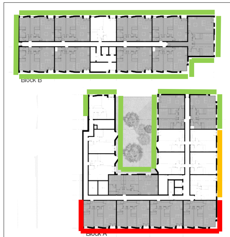
Plan Showing Façade Performance Zones – Level 01-02
