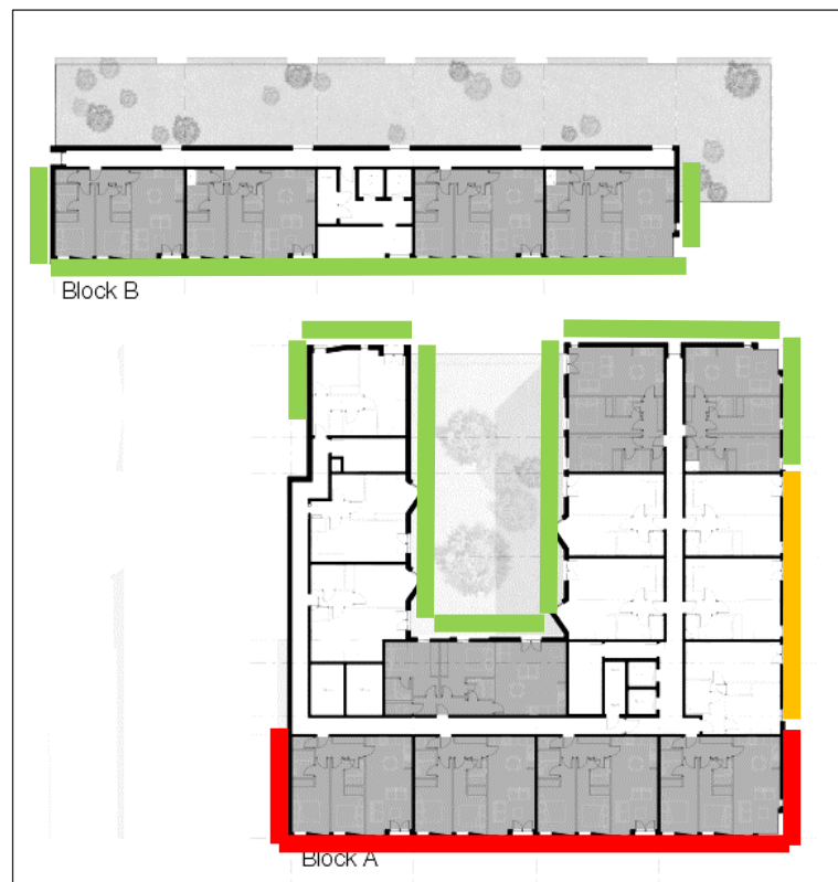
Plan Showing Façade Performance Zones – Level 03
