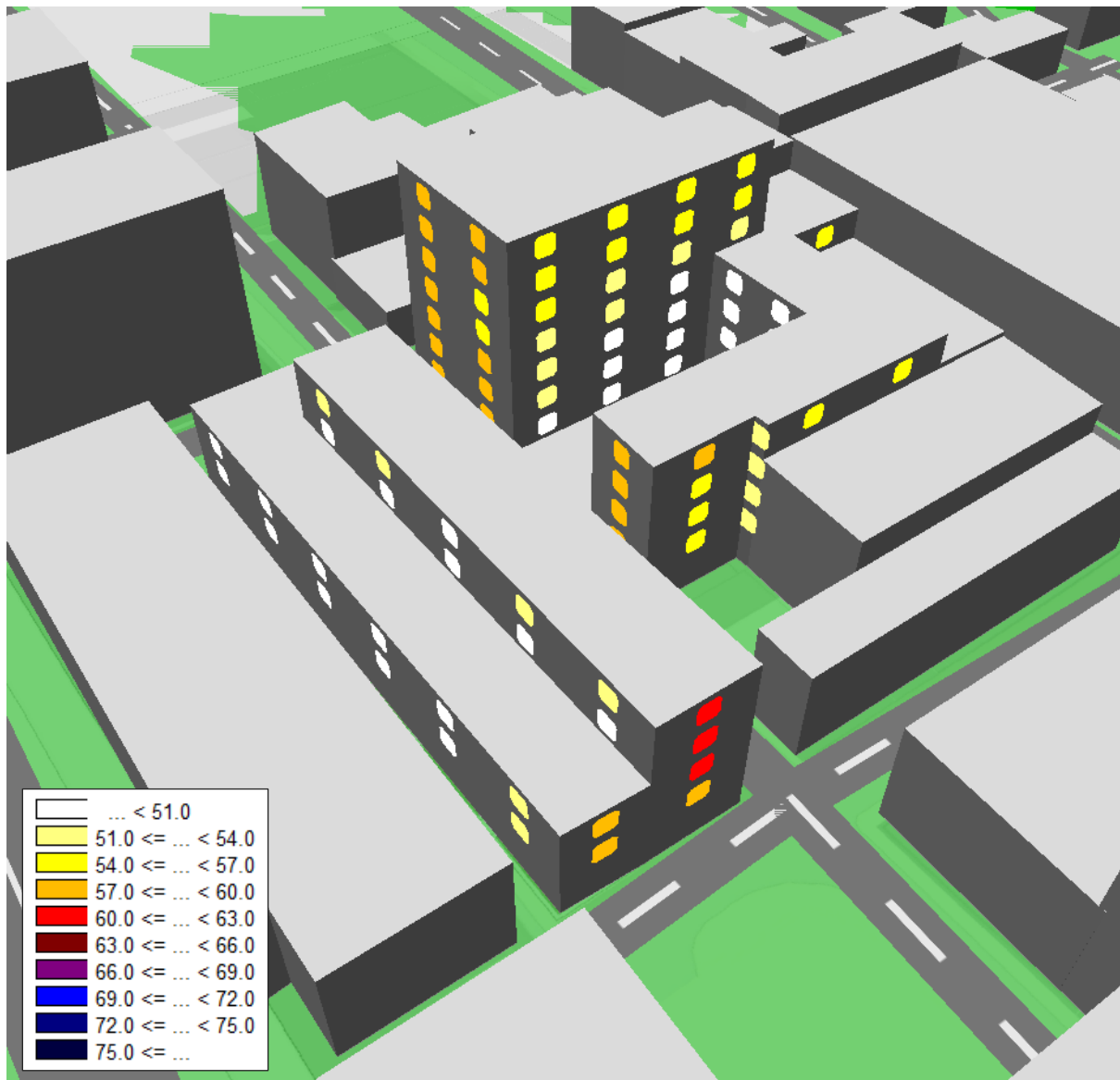
Daytime Incident L_{Aeq,16hr} Noise Levels (from east)
