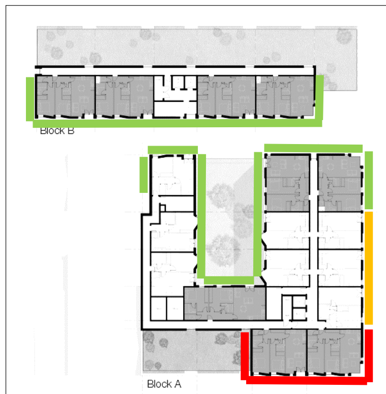
Plan Showing Façade Performance Zones - Level 04-05
