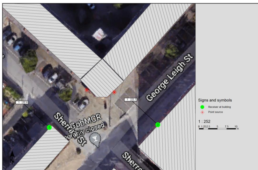
Figure 6: Noise Breakout Through Facades, SP Overview
