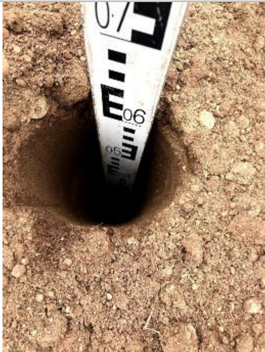
Depth of Cover System at Ground Level
