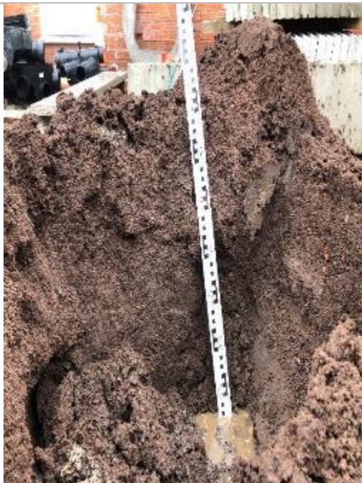
Depth of Cover System at Ground Level
