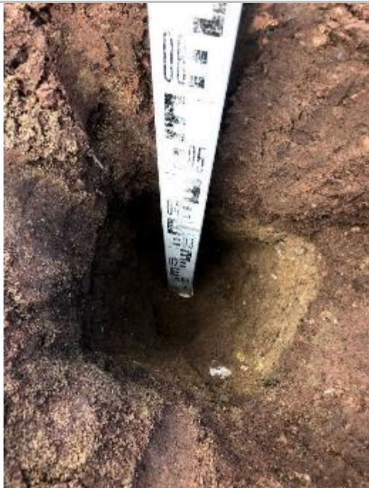
Depth of Cover System at Ground Level
