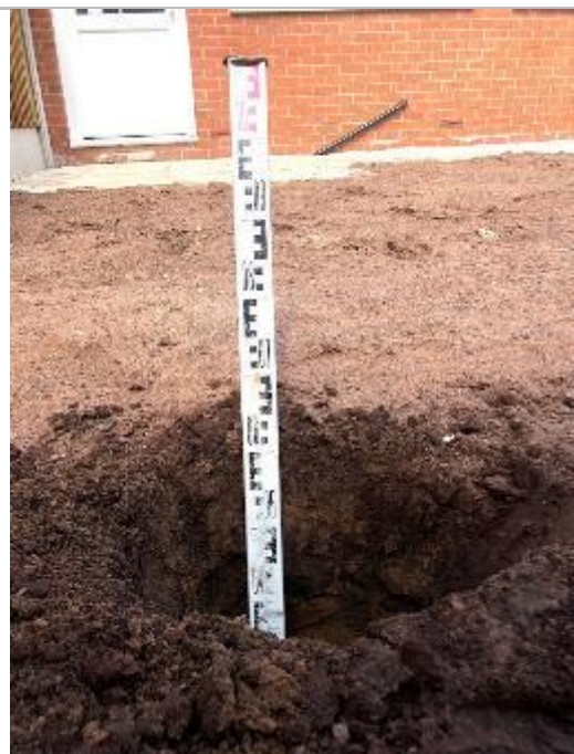
Depth of Cover System at Ground Level
