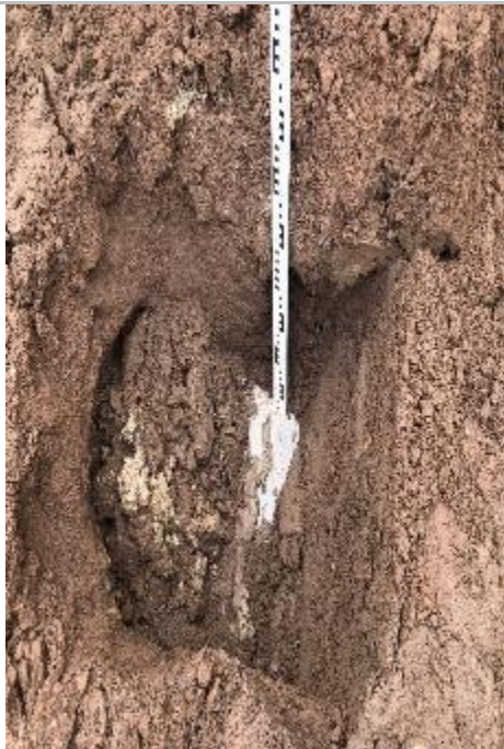
Depth of Cover System at Ground Level
