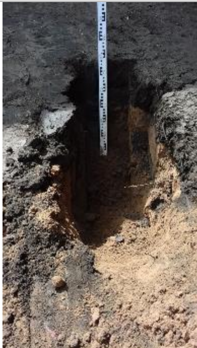
Depth of Cover System at Ground Level
