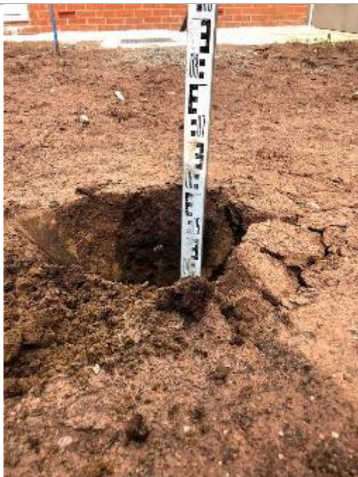
Depth of Cover System at Ground Level
