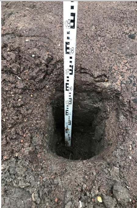
Depth of Cover System at Ground Level
