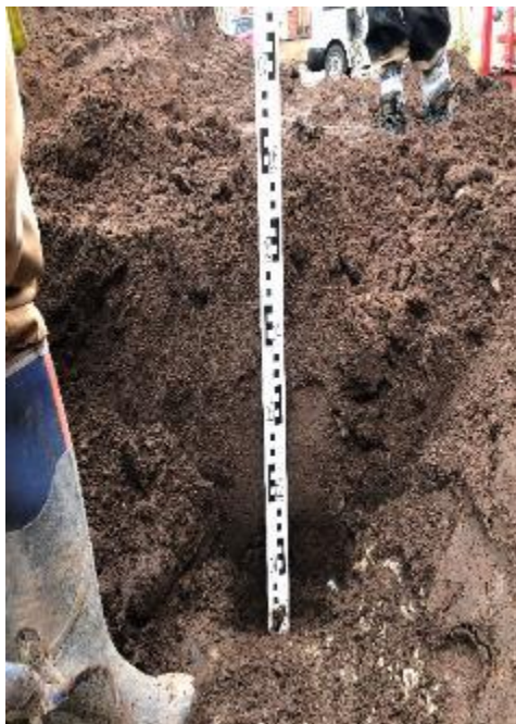
Depth of Cover System at Ground Level
