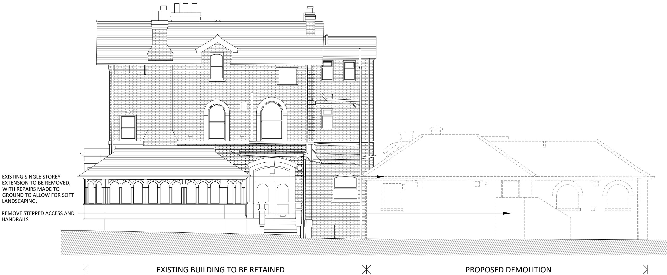
03 PROPOSED SOUTH WEST ELEVATION 070 SCALE - 1:100@A1 DEMOLITION
