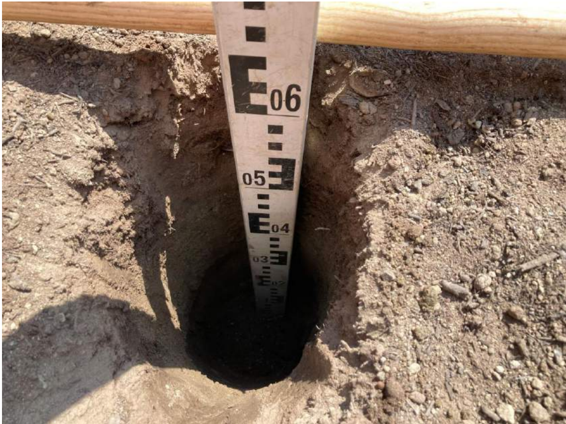
Photograph 7 150mm of topsoil and 450mm of subsoil emplaced in VP04.
