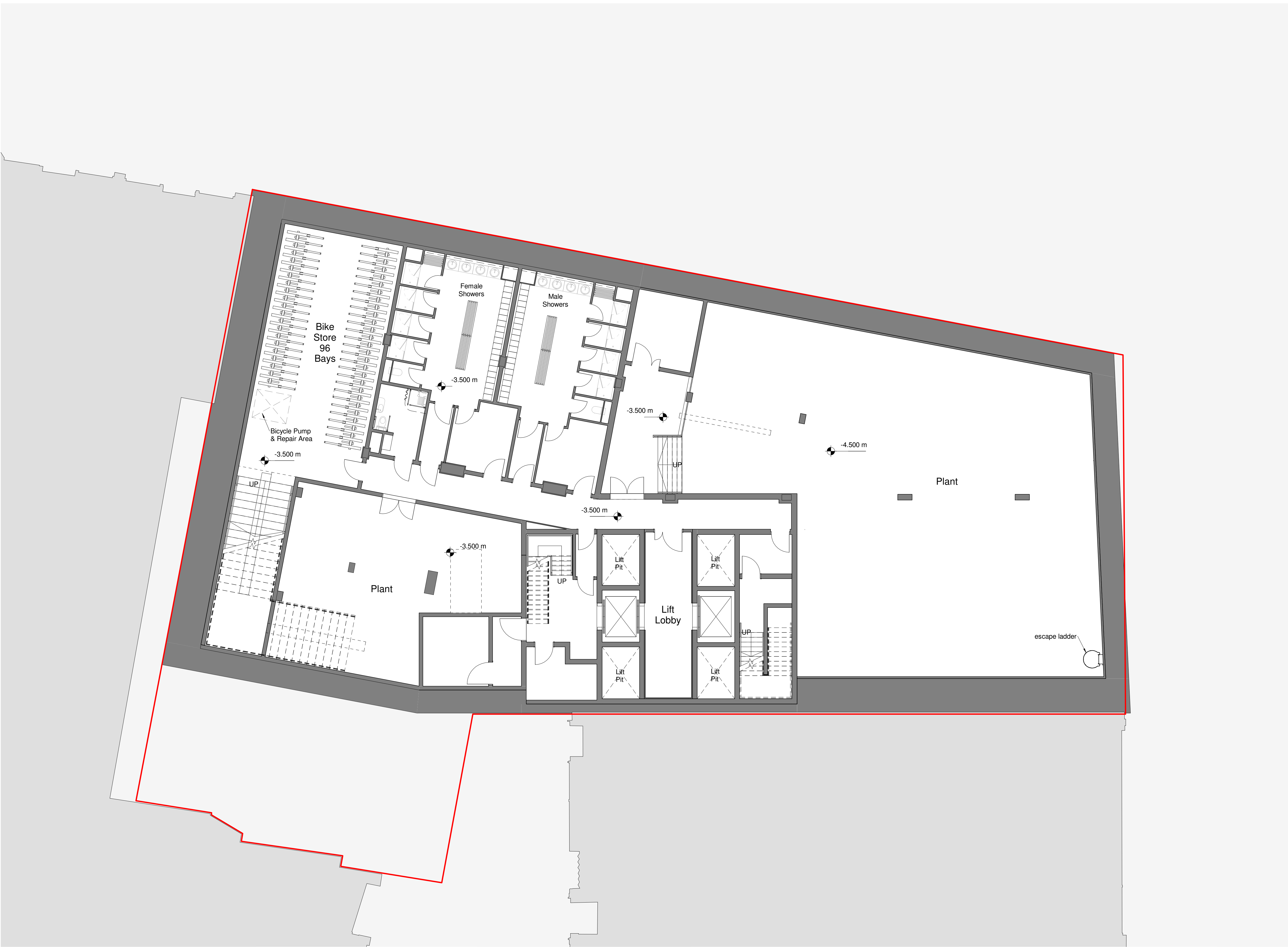
Proposed Basement Plan 1 : 100
