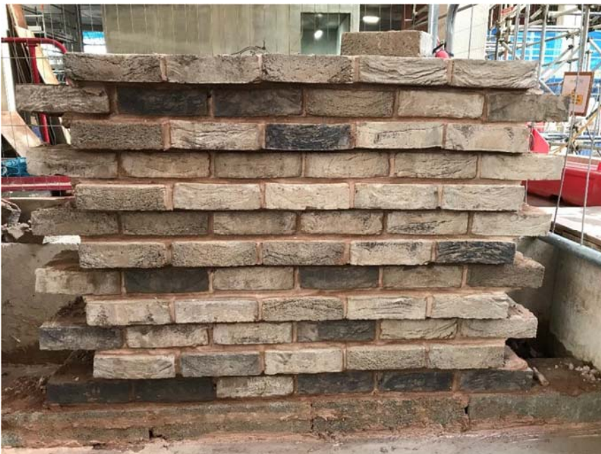
Projecting brickwork with a approx. 25mm projection
