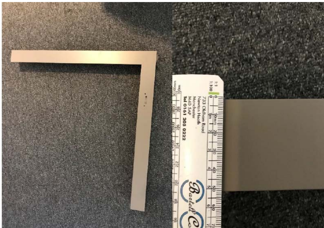
Powder coated (RAL7006) window frame sections showing a 50mm elevational / front face
