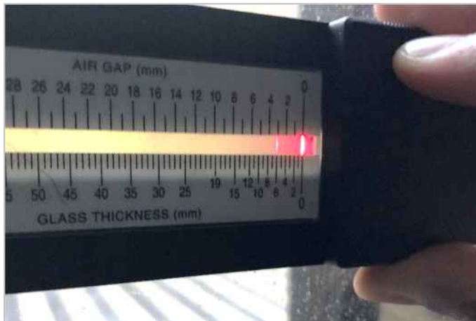
Photograph No. 12 – 6mm glazed pane measured
