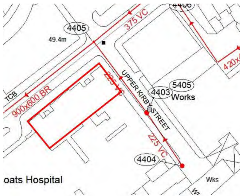
Figure 2: Extract from UU Sewer Records (2006)
