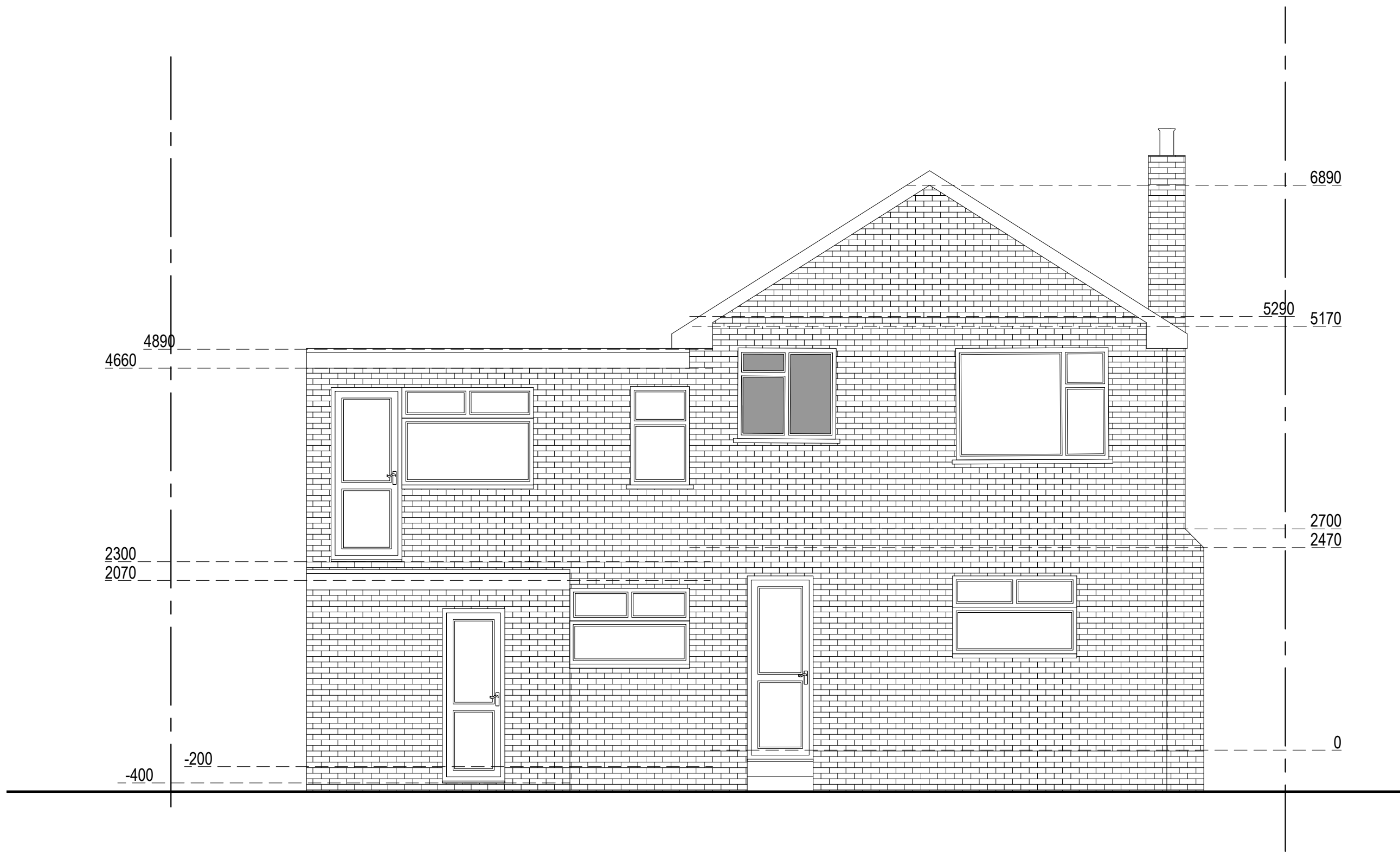
Existing Southwest Elevation Scale 1:50
