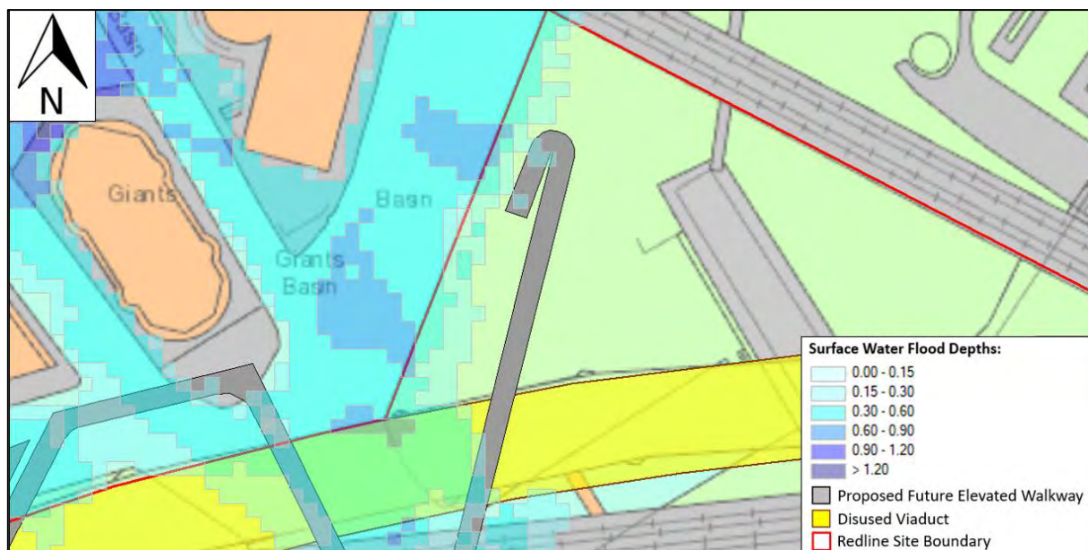
Figure 4-8: EA 1 in 1,000 Year RoFSW Flood Depth and Flood Extent Map (Source: Environment Agency)
