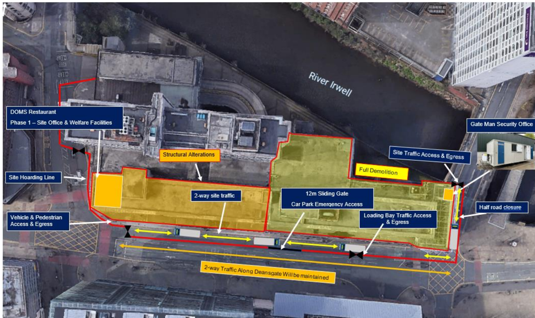
Figure 1 shows the access / egress points at the site for the demolition phase
