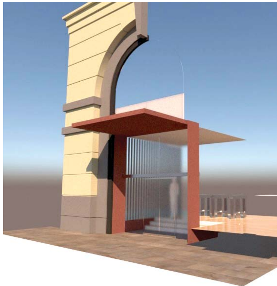
CGI of canopy insertion into existing opening
