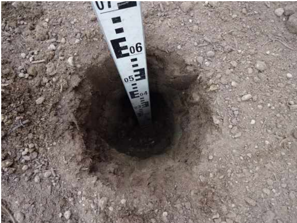
Photograph 4 Plot 5 rear garden with 600mm capping.
