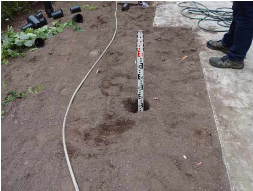
Photograph 3 Plot 5 rear garden with 600mm capping.
