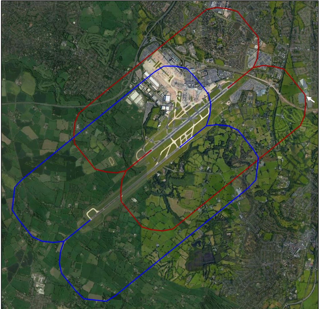
Figure 11 Circuits paths for runways 05L-23R (red line) and 05R-23L (blue line)
