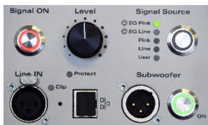
Control panel of PA3 Power Amplifier
