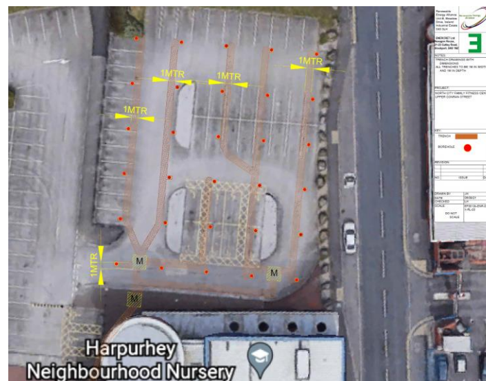
Figure 4 - Borehole and Trenching Layout
