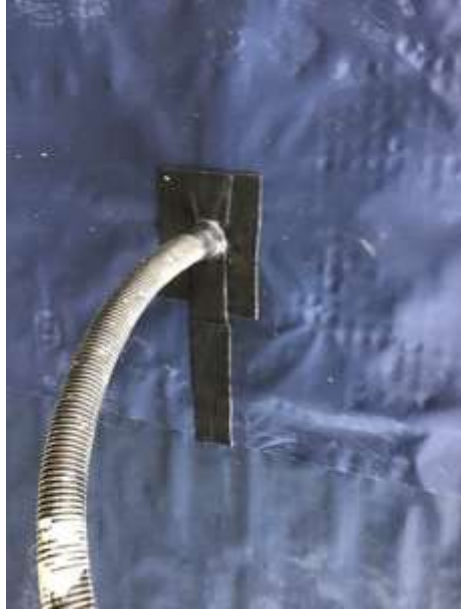
Pipe seal being pick tested
