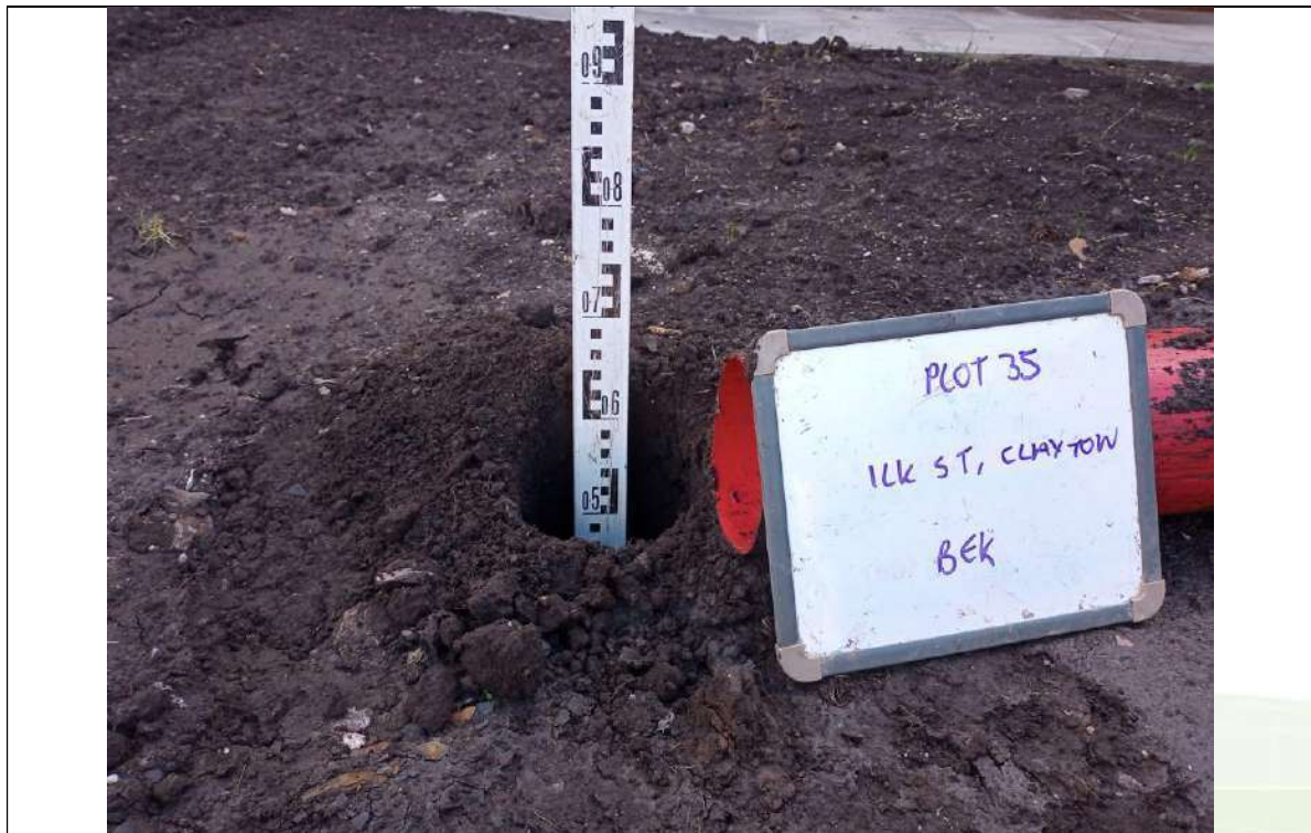
Photograph 1: Validation of Garden Capping Thickness
