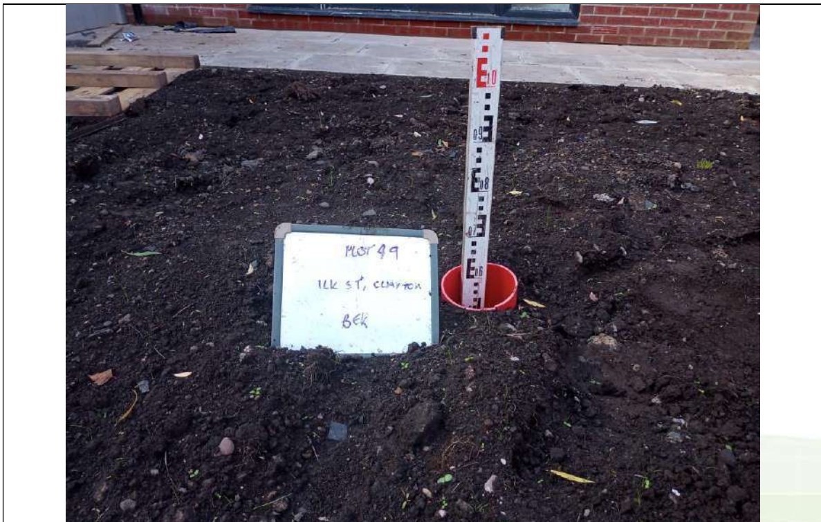
Photograph 1: Validation of Garden Capping Thickness
