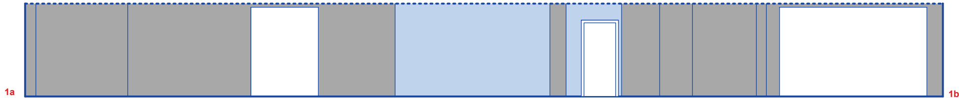
PART-INTERNAL (UP TO PITCH CHANGE) ELEVATION OF SPINE WALL 1-1: WALLS ARE COLOUR CODED TO DELINEATE BETWEEN EXISTING AND PROPOSED WALL TYPES
