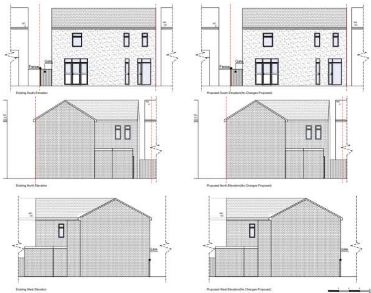
Figure 3: Existing and Proposed Site elevations
