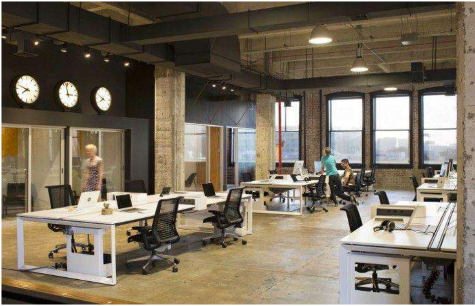
Industrial trunking for power and lighting distribution, exposed cable trays and ductwork, bench office furniture, exposed joists in certain areas.
