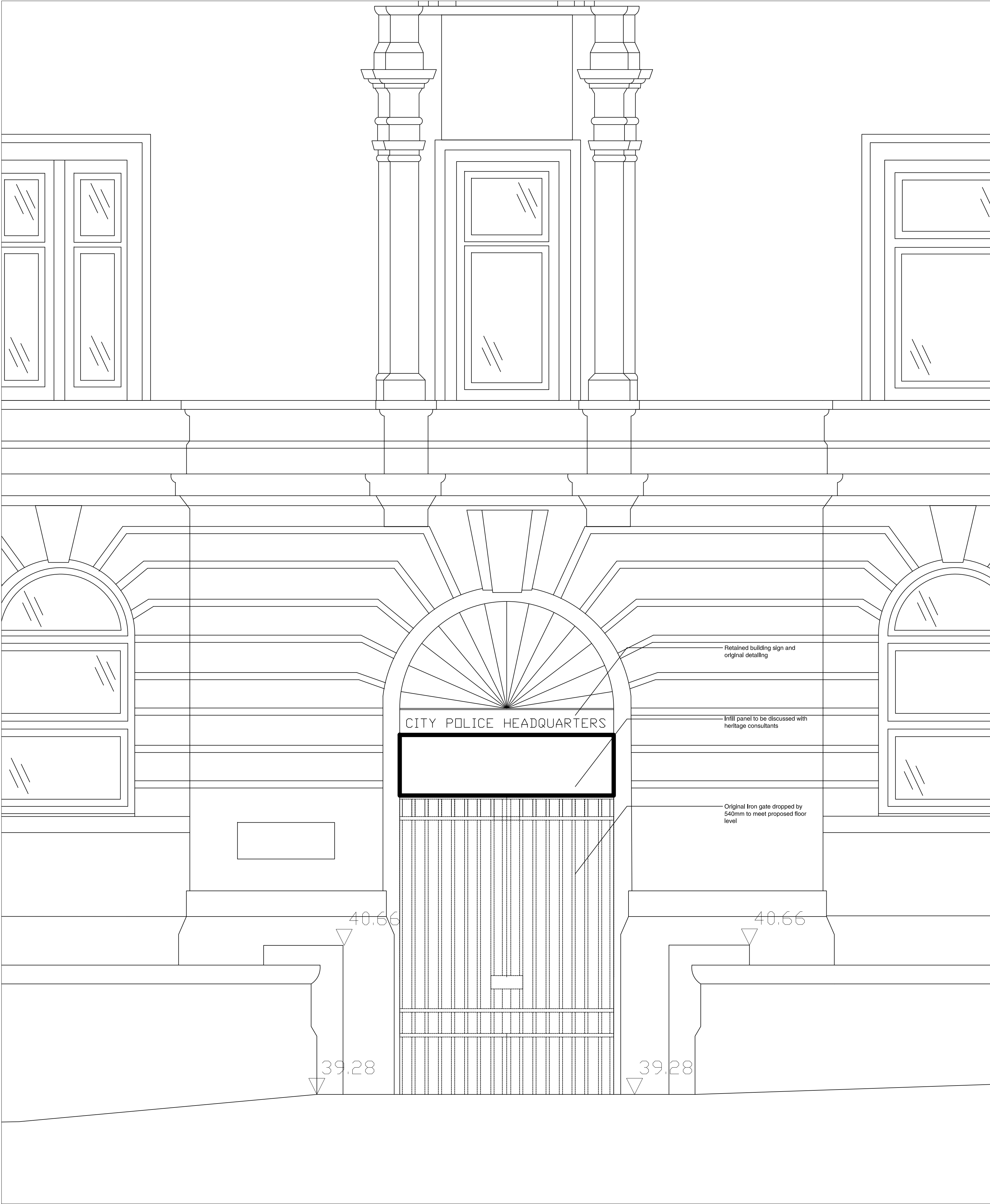
1 GA Planning - Police Station Elevation 1 : 20
