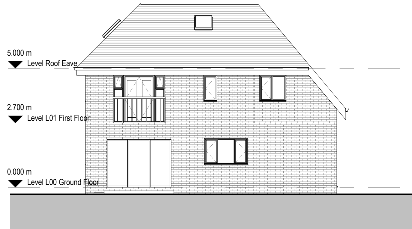
3 Existing West Elevation 1 : 100
