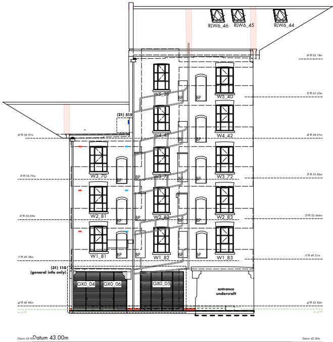
proposed courtyard elevation 3 undercroft to building 2
