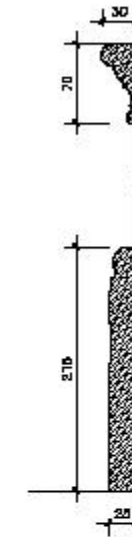
4 - SKIRTING & WALL PANEL MOULDING 1:10
