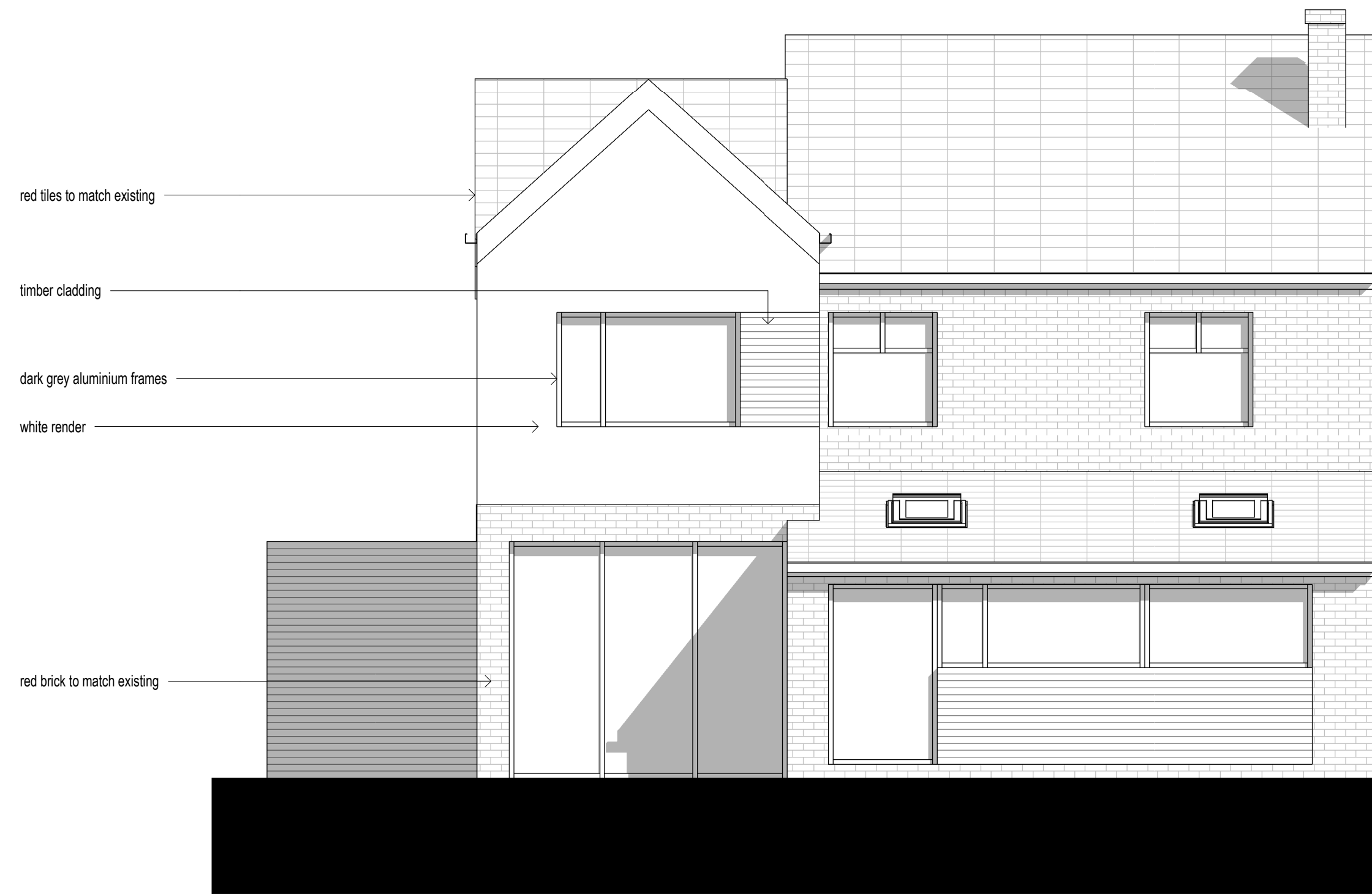
North Facing Elevation
