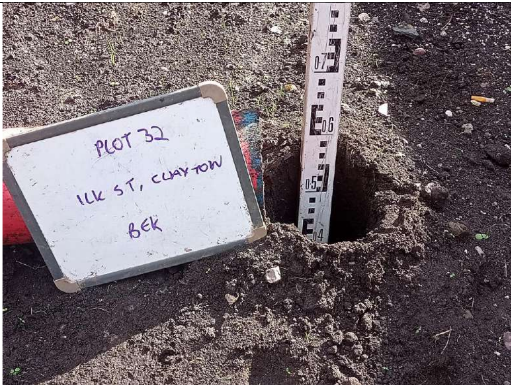
Photograph 1: Validation of Garden Capping Thickness
