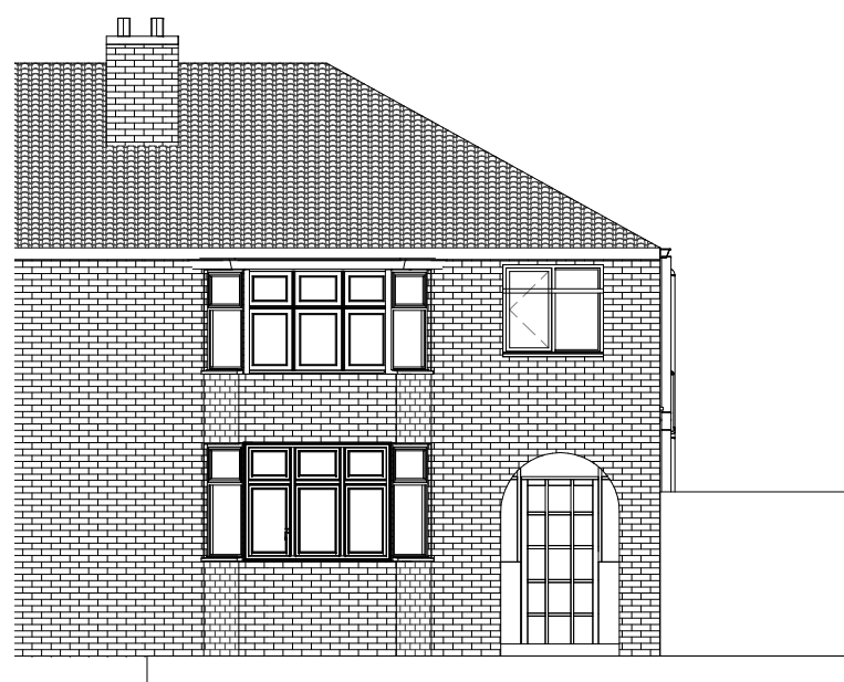
Existing Front Elevation 1 : 100
