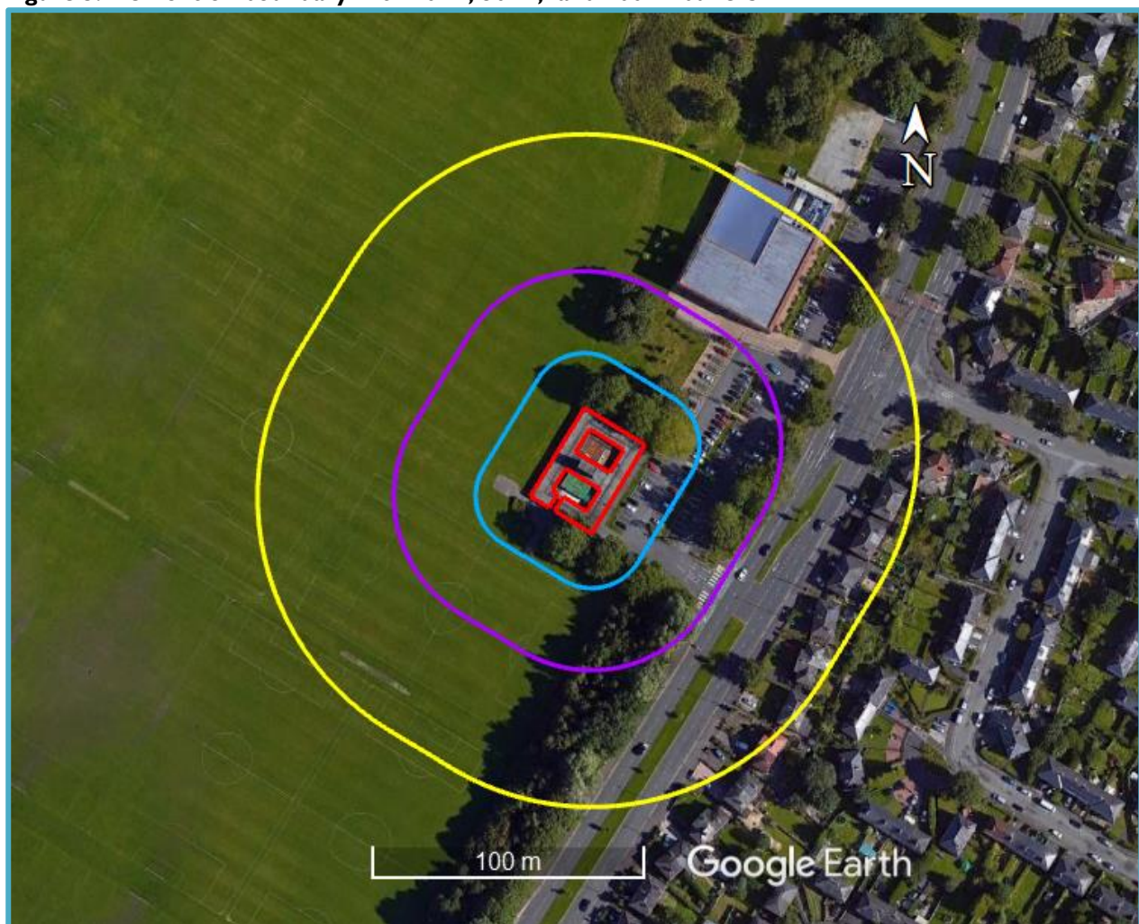
Figure 3. Demolition boundary with 20 m, 50 m, and 100 m buffers
