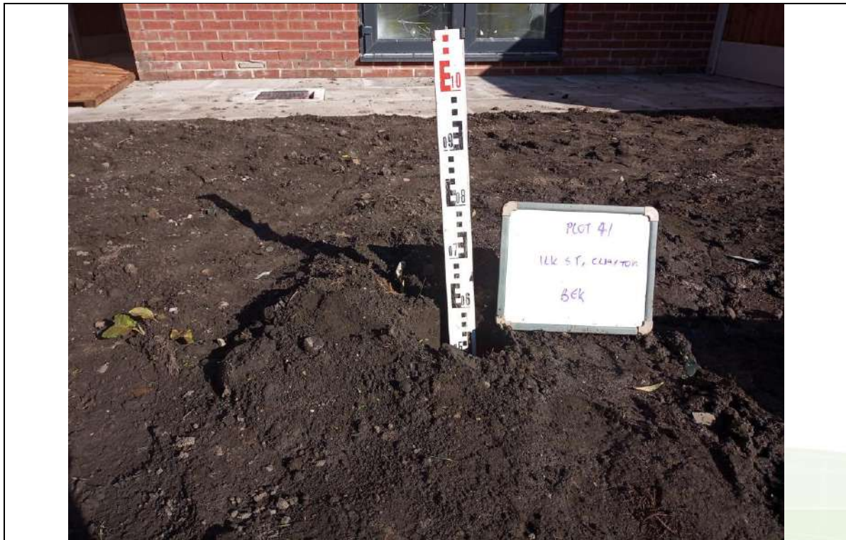
Photograph 1: Validation of Garden Capping Thickness
