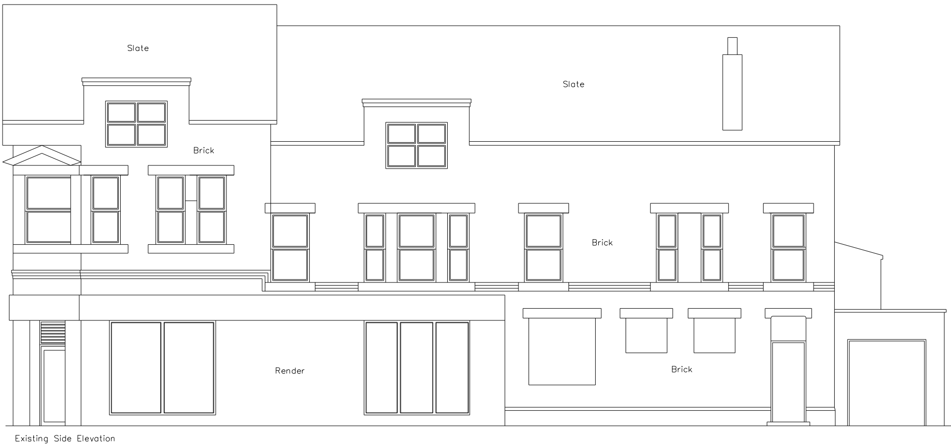
Existing Side Elevation
