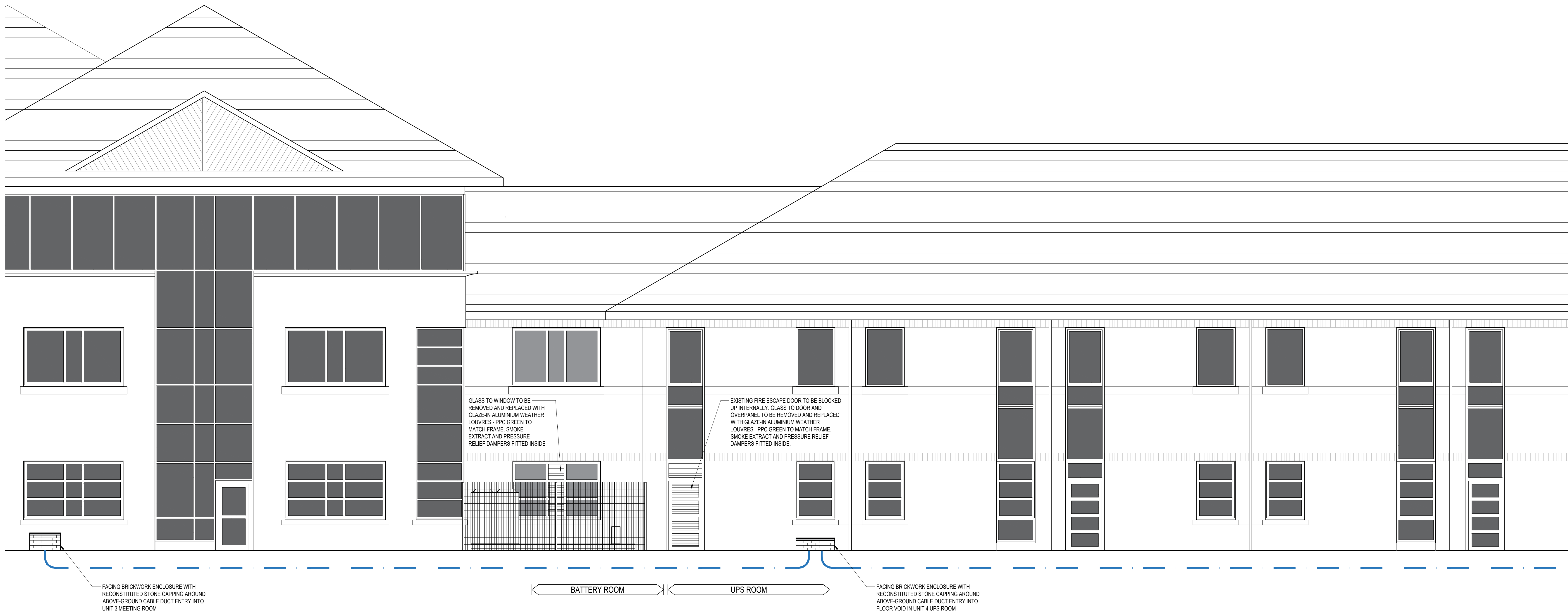
2 WILLIAMS HOUSE NORTH ELEVATION (PARTIAL) SCALE: 1:50 @ A0
