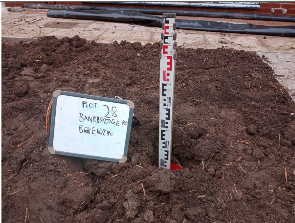
Photograph 2: Validation of Garden Capping Thickness
