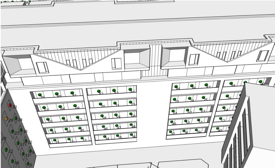
Figure 4 – VSC to B1: south facing elevation to court yard
