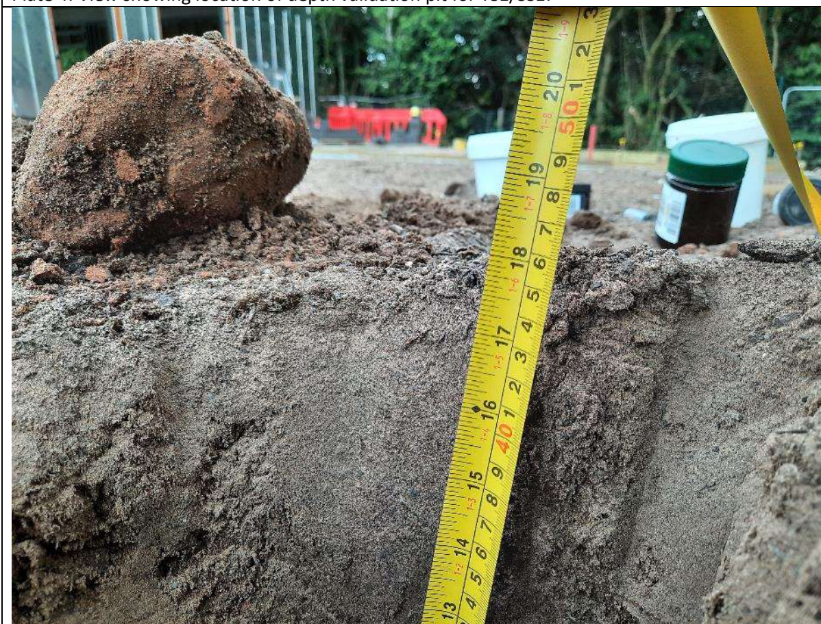
Plate 5: View showing depth of imported material at TS1/SS1.
