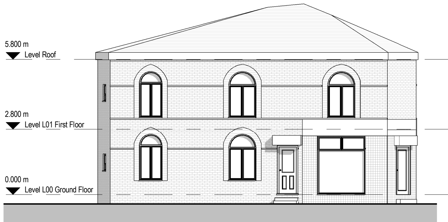
2 Existing North Elevation 1 : 100
